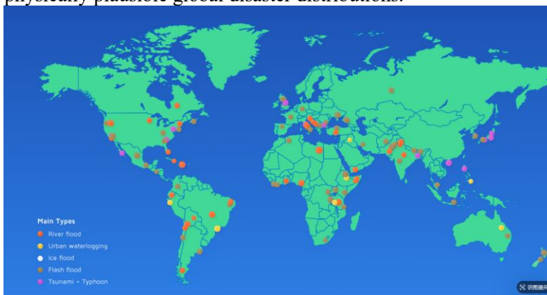
Figure 2: Global distribution of detected water-related disaster events; Each point represents an individual event identified through the proposed framework, with colors indicating major hazard types.
