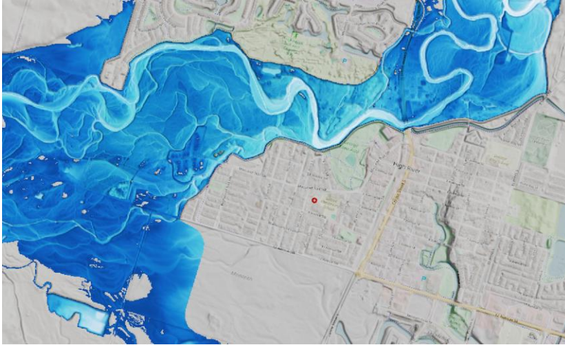
Figure 3: Example of simulated fluvial flood depths for return period 1 in 100 years, close to High Rivers with all design protection included in simulation
