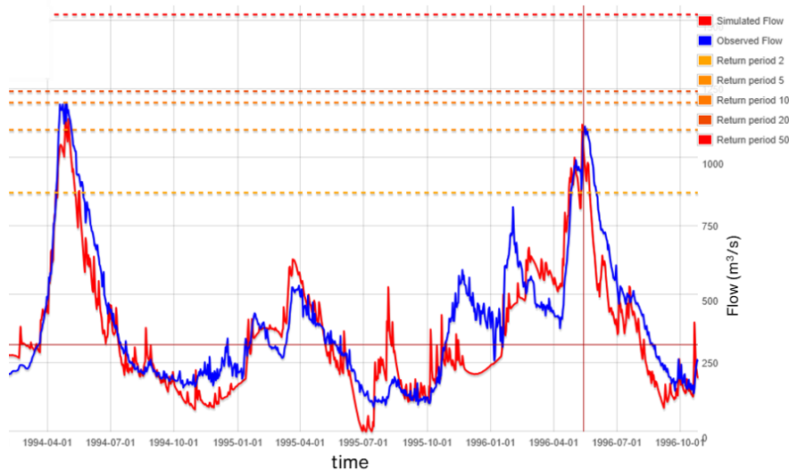
Figure 2: Example of HYPE–mizuRoute calibration at a selected HYDAT gauge, showing observed and simulated daily discharge and demonstrating the ability of the model to reproduce seasonal regimes and high-flow events.
