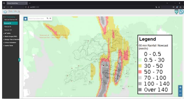
Figure 5 – Screenshot of M 3 's user interface accessed through web browser, showing the city-wide layers of modelled flood extent, forecasted rainfall contour, predicted tide levels and flood extent at one glance
